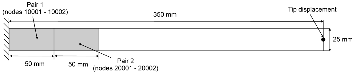
Figure 8.11: Cantilever beam with two pairs of piezoelectric patches
